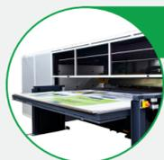
The suction cups of the loader system are divided by groups, which makes possible to load automatically, and **print up to 6 separated substrates at the same time**.
